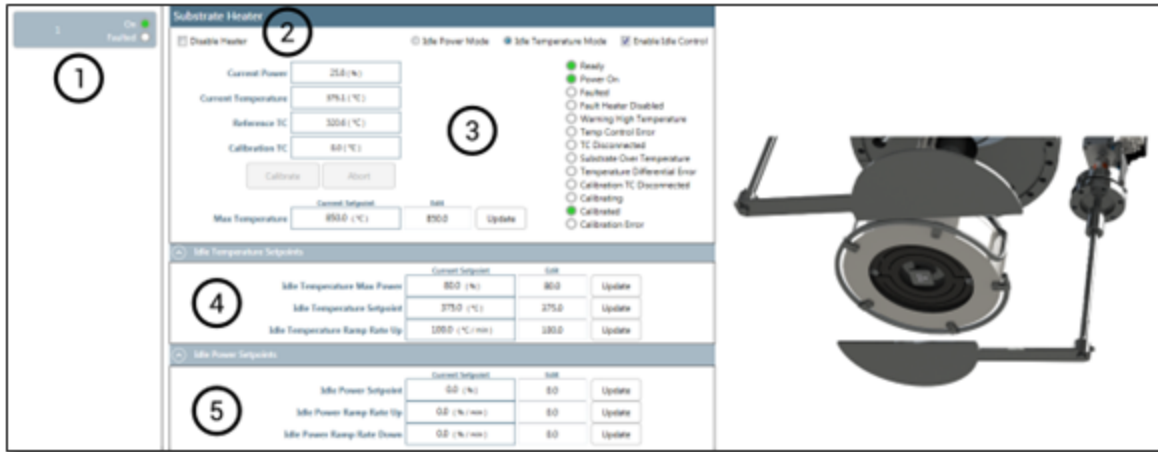
The Heaters Page provides the Aeres ® user with access to temperature and power controls
