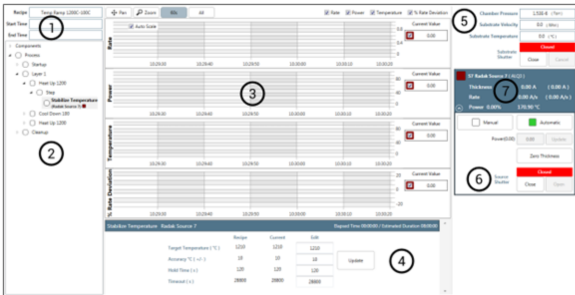
Structure of the Process Page, providing real-time monitoring of the deposition
